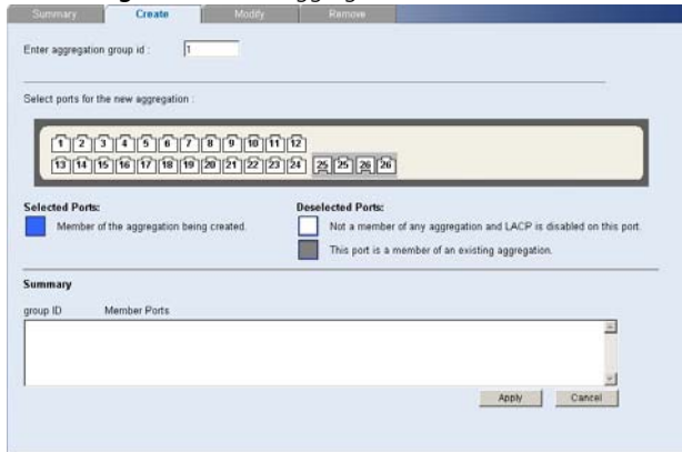
Figure 41 Link Aggregation Create Screen
